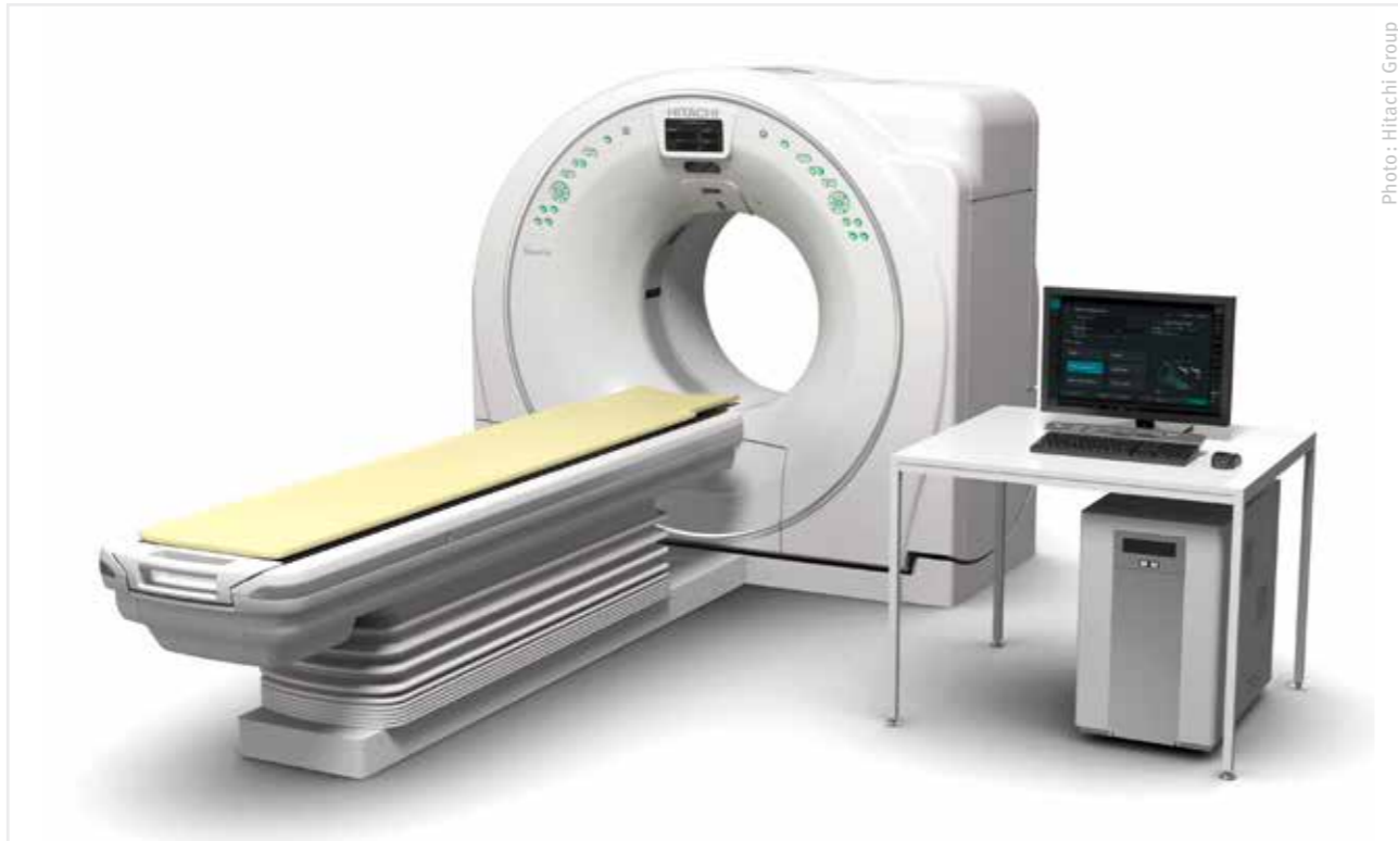
Equipped with 64 rows of X-ray detectors, the Supria 64 CT system scans broad areas at high speed. Compared to its 16-row predecessor released in 2007, the latest model achieves annual power savings of roughly 60% during use.
